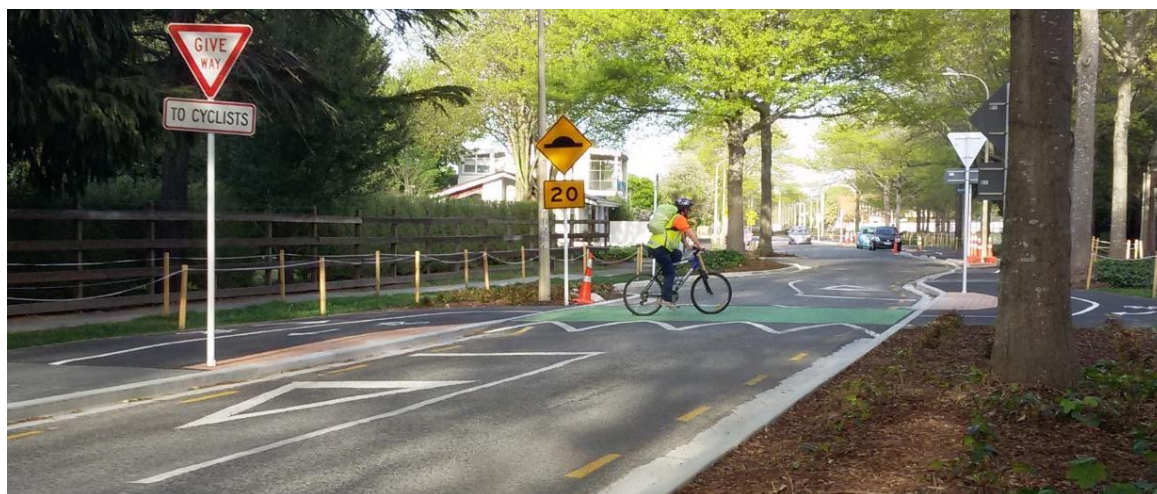
Figure 69: Supplementary ‘to cyclists’ plate on give way sign at midblock priority cycle crossing, Uni-Cycle route, Christchurch
