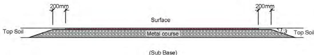
**Figure 27: Cross section for chipseal or AC path without timber edging battens**
