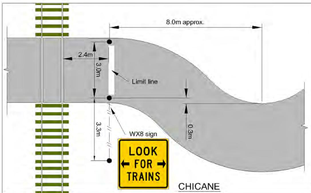
Figure 46: Chicane design; slows cyclists before crossing railway line
