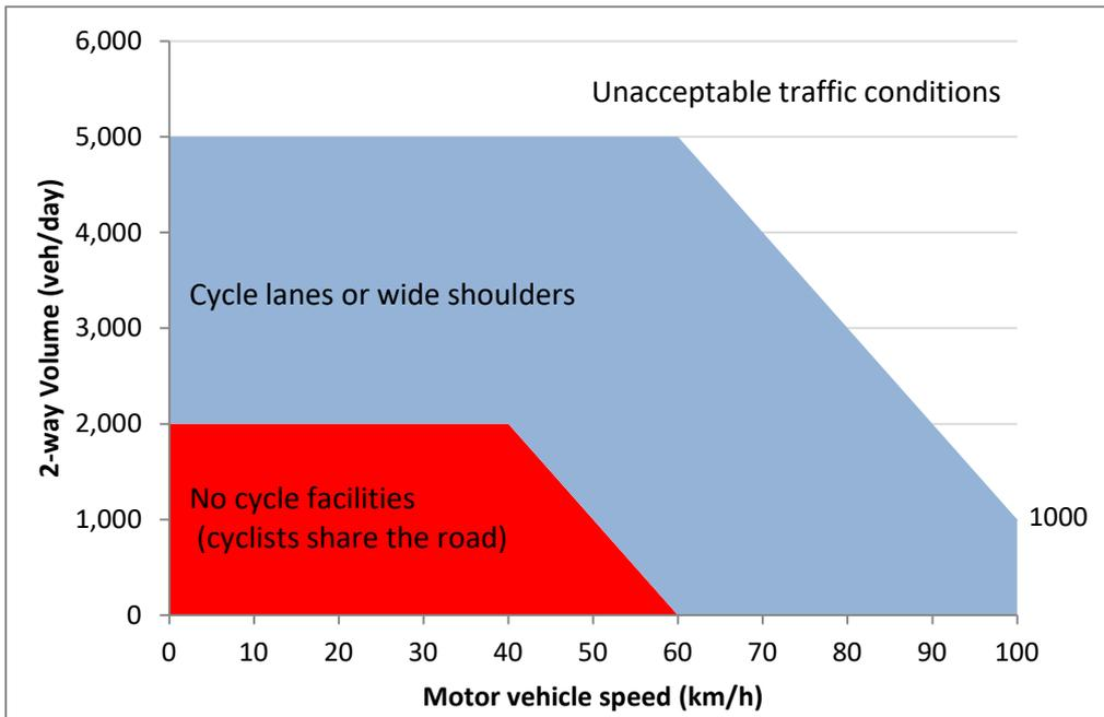
Figure 33: Trail type for Grade 1 and 2 on-road trails
