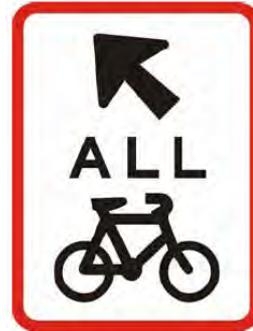
Figure 74: All cyclists must exit regulatory sign (RG-26b) (Transit NZ, 2008b)
