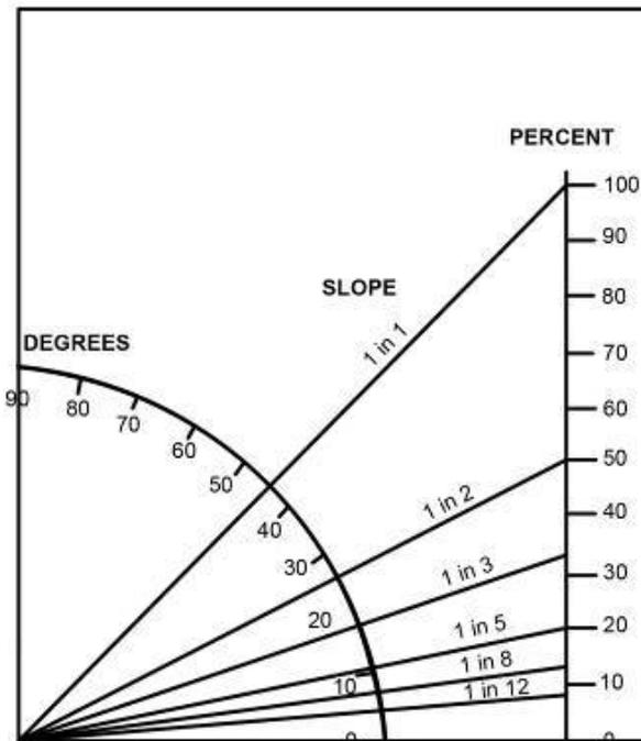
Figure 15: Relationship between degrees, percent and slope
