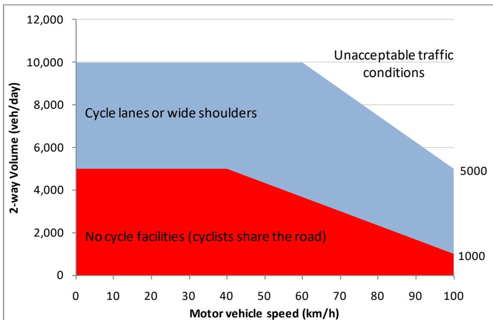
Figure 34: Trail type for Grade 3 and 4 on-road trails
