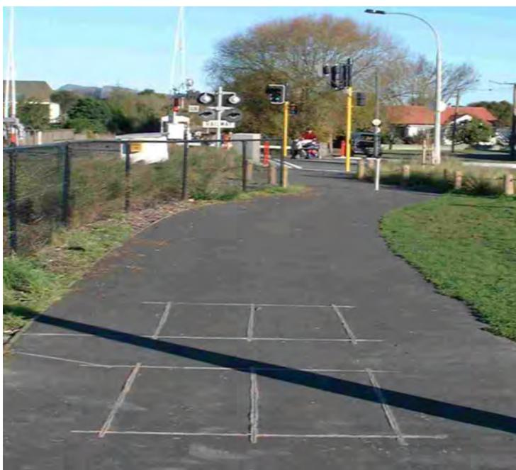
Figure 41: Advance cycle detection for signals, Railway Cycleway, Christchurch
