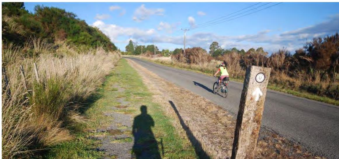
**Figure 9: Poorly-surfaced cycle paths next to low-volume roads will not be used by cyclists**
